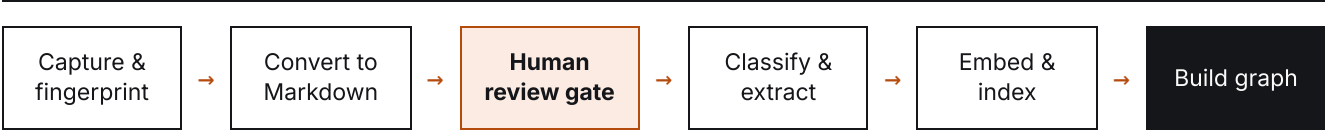
FIG. 1 The ingestion pipeline. Each step records when it completed. Nothing is embedded or added to the graph until the review gate is passed.
